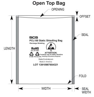
Tolerance: Width -0, +1/4" Length +/- 1/8" Offset 0 to 1/4" Seal width 3/8" with a tolerance of +/- 1/8"
