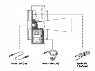
Be sure to ground the 50B-S series enclosure to ensure the stable performance of the product and avoid electric shock.
