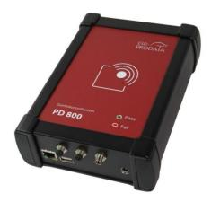
At ESD test stations, the results of the personal tests are to be stored and archived. This happens at many test stations over handwritten entries in lists and therefore costs time. The archiving of these lists requires paper, effort and also time. The PD-800 acquisition system takes care of the complete acquisition and archiving and can be connected to almost every personal tester via the potential-free signal inputs.
