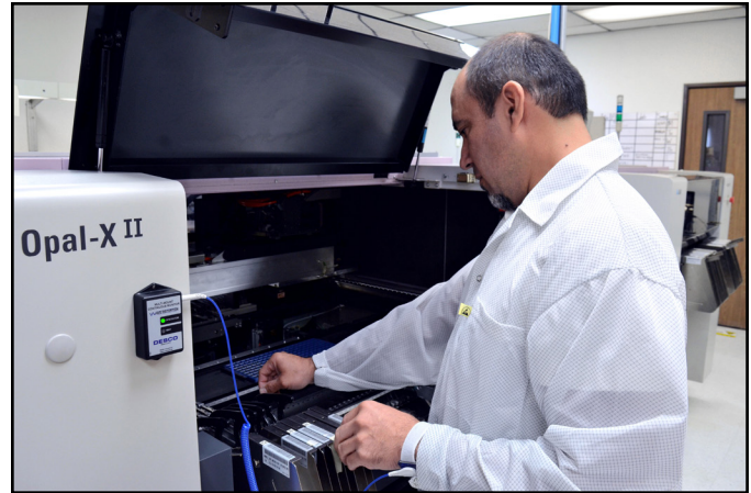
Figure 11. Using the Multi-Mount Monitor at a machine station
