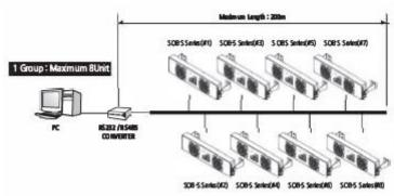
The method of connecting to the computer with multi-port
